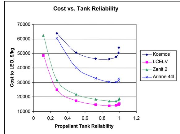
**Figure 7. Cost Reduction vs. Propellant Tank Reliability**
