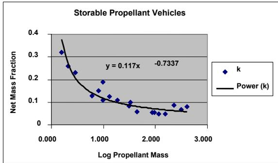
**Figure 5. Net Mass Fraction for Storable Propellant Vehicles**
