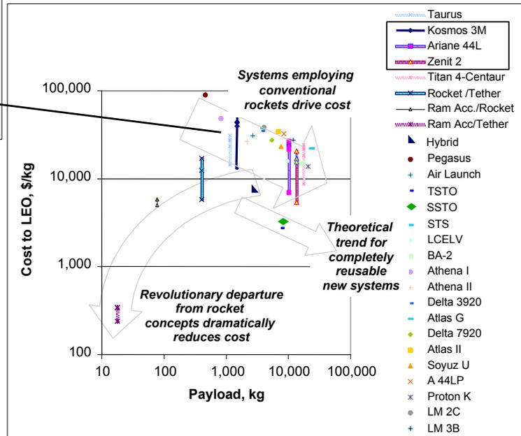
Figure 12. Launch Costs to LEO vs. Payload
