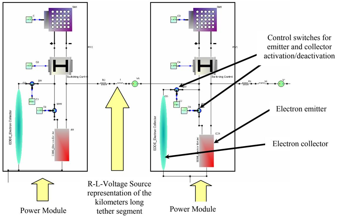
Figure 6. Configuration of single tether segment in VTB
