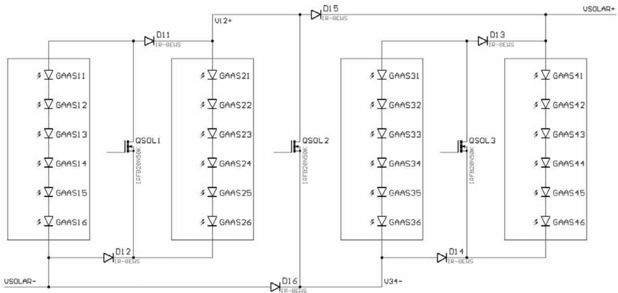
**Figure 4. Series/parallel switching of 4 solar array strings**
