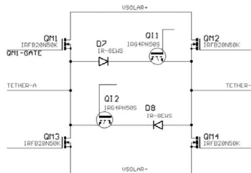
**Figure 3. Opto-Isolated gate drive circuits, and H-bridge with IGBT-controlled shunts**
