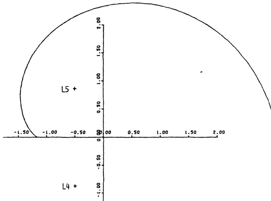
FIG. 10. Orbit of Small Body Released Near L2 with Small Velocity Away from the Moon
