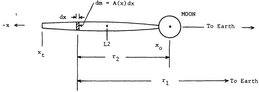
FIG. 3. Notation for Anchored Lunar Satellite Problem
