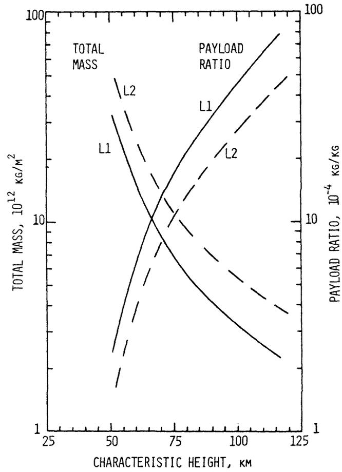
FIG. 8. Mass and Payload Capacities for Lunar Anchored Satellites
