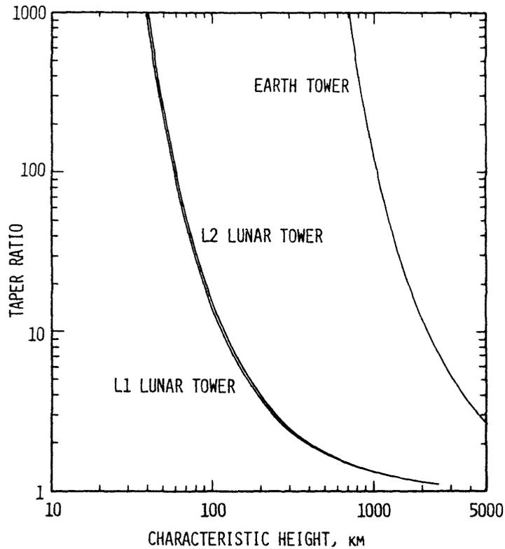
FIG. 5. Taper Ratios Required for Anchored Lunar Satellites
