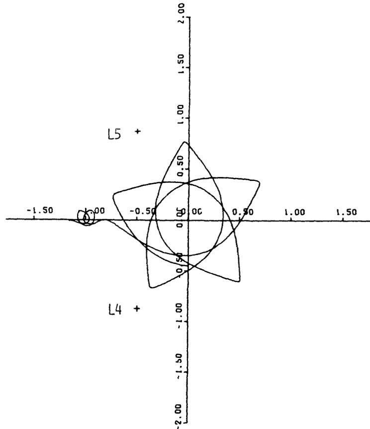
FIG. 9. Orbit of Small Body Released Near L2 with Small Velocity Toward the Moon
