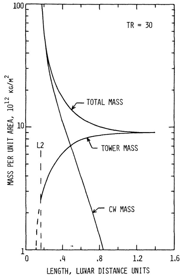
FIG. 7. L2 Lunar Satellite Mass and Counterweight
