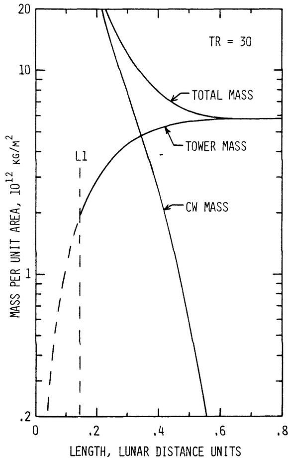
FIG. 6. L1 Lunar Satellite Mass and Counterweight
