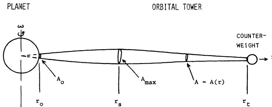
FIG. 1. General Features of an Orbital Tower
