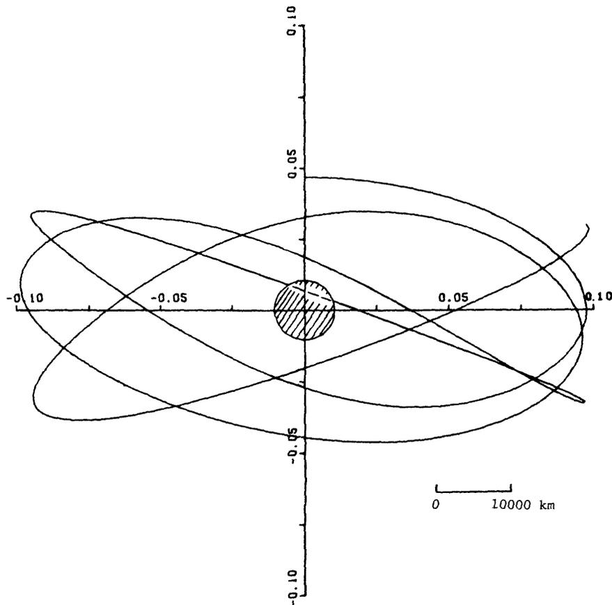
FIG. 15. Example Path of Anchored Lunar Halo Satellite Seen from L1
