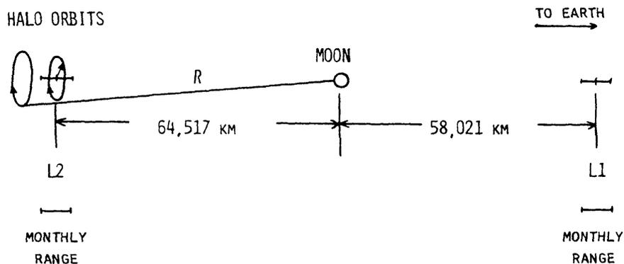
FIG. 13. Lunar Halo Orbit for Farside Communication
