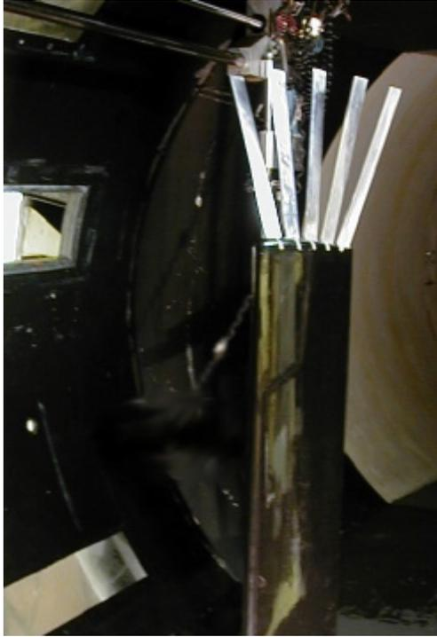
Figure 1. Wing model with winglets
