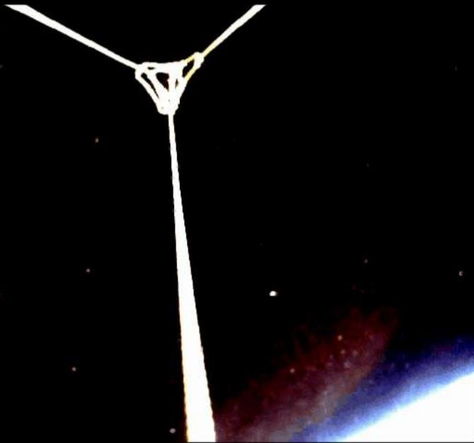
Spin up test of hanging bead-chain net
